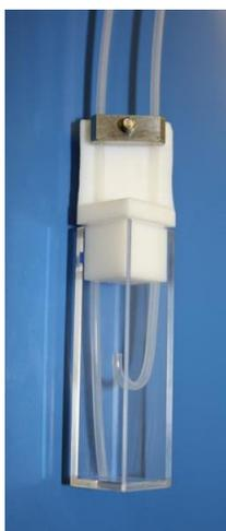
Figure 3.8: position of the tubing within the sample cell
