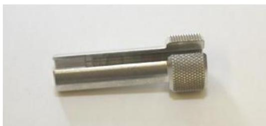
Figure 3.5: flow tubing tightening tool
