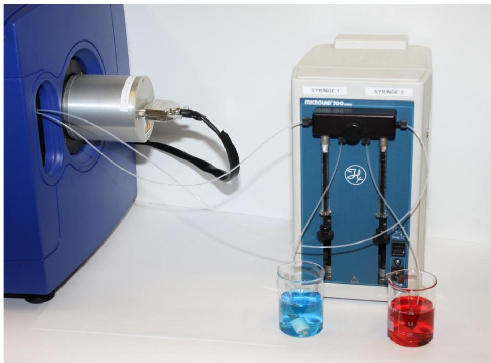
Figure 3.11: the fully assembled CS/TT accessory
